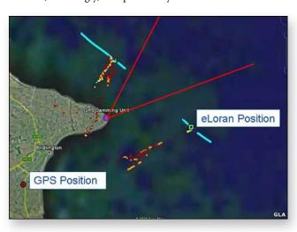
In the UK trial. GPS in the jamming zone (red triangle) reported positions tens of km away from the true (eLoran) position. Courtesy, BBC
