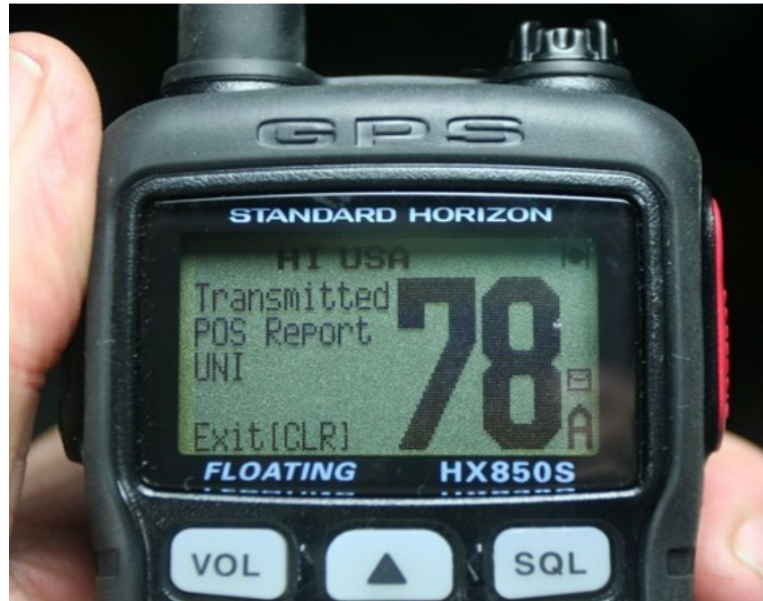
Screen of Standard Horizon 850S DSC Radio, in use by many Division 10 Aux Aviators, shows Position Report (or Distress Signal) sent, complete with MMSI number and GPS location.
