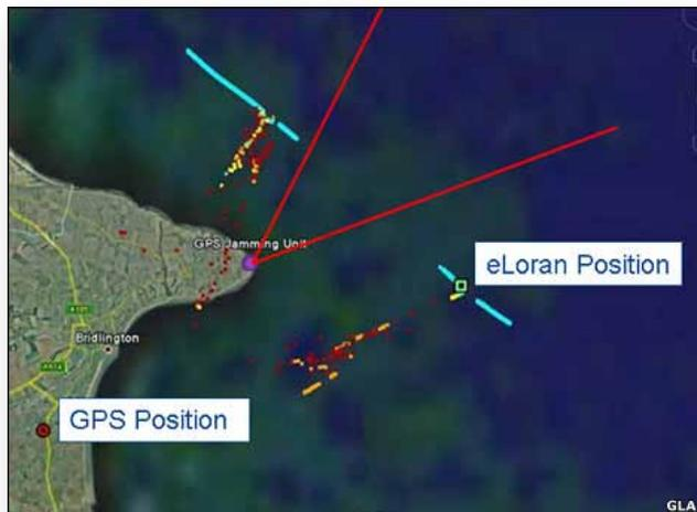
In the UK trial, GPS in the jamming zone (red triangle) reported positions tens of km away from the true (eLoran) position. Courtesy, BBC
